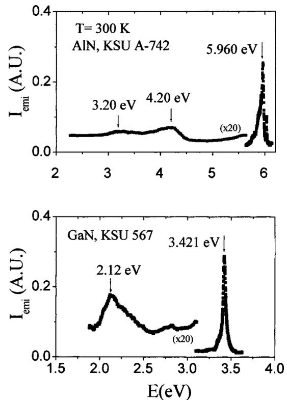
FIG. 2. PL spectra of AlN and GaN epilayers measured at 300 K, which covers a broad spectral range.
