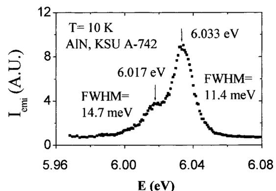
FIG. 3. Edge-emission spectrum of AlN measured at 10 K.
