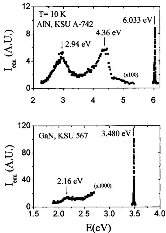
FIG. 1. PL spectra of AlN and GaN epilayers measured at 10 K, which covers a broad spectral range from 2.2 to 6.2 eV for AlN and 1.8–3.6 eV for GaN.
